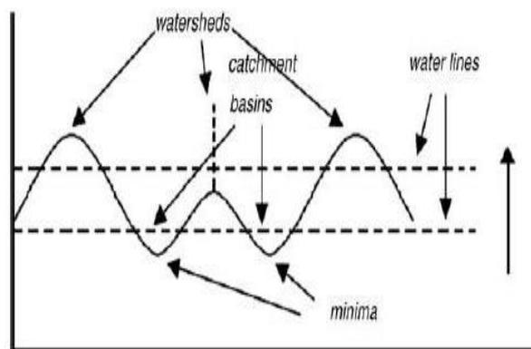
Fig. 1. Watersheds and Catchment basins. Basins are defined as connected regions with local minimum to which any incident rainfall will flow.
